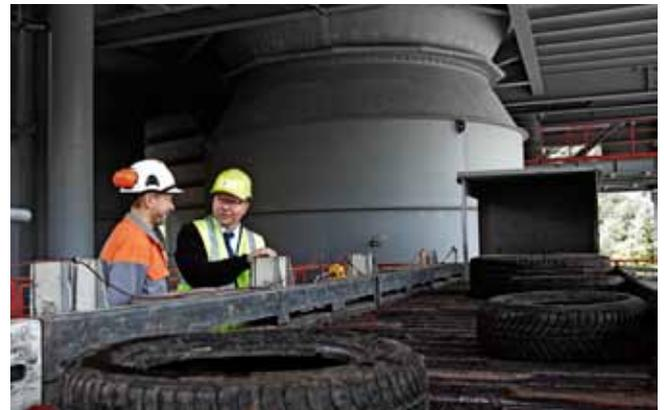
The HOTDISC™ is capable of treating alternative fuel in all shapes and sizes – in Anhovo’s case, whole tyres.
