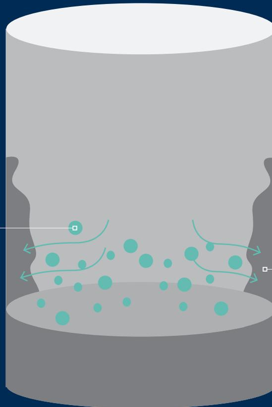
**2. Prehydrated cement on the silo wall**
