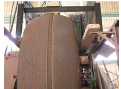
Grinding roller after repair
