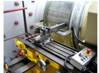
Press polishing of trunnion
