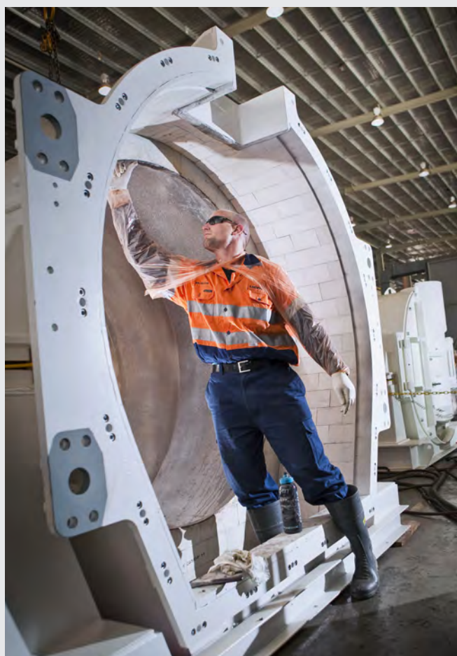
Applying WEAR MAX® to centrifuge housing
