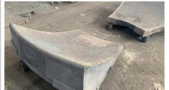
OK™ Pro+ wear liners are currently available for rollers and tables of all OK™ raw mills and most OK cement mills with full roller segments.
