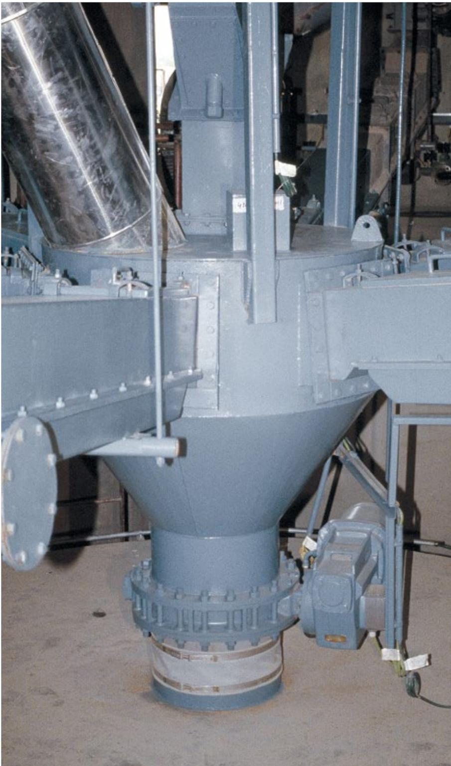
Each of the seven outlets is provided with a shut-off valve by which extraction from a given outlet can be started and stopped together with the aeration of the appertaining segments. Slide gates are provided to facilitate the maintenance of the shut-off valves.
