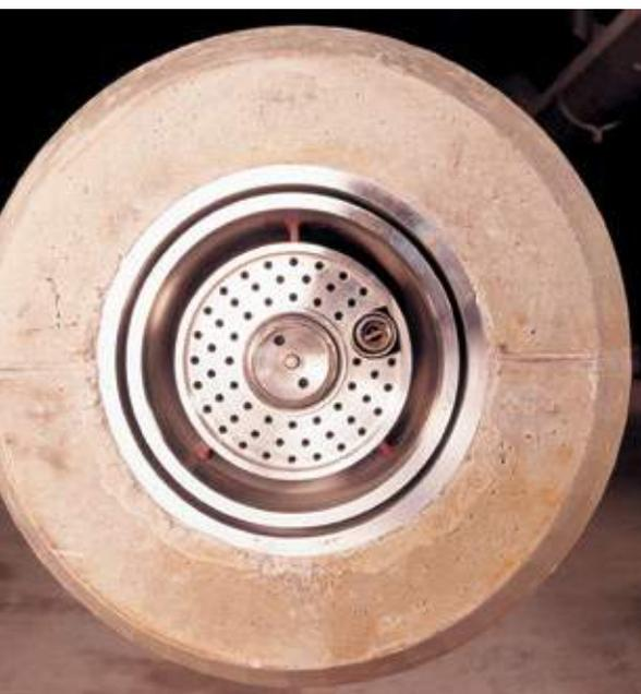
A constant momentum can only be maintained by adjusting axial air as well as swirl air.
