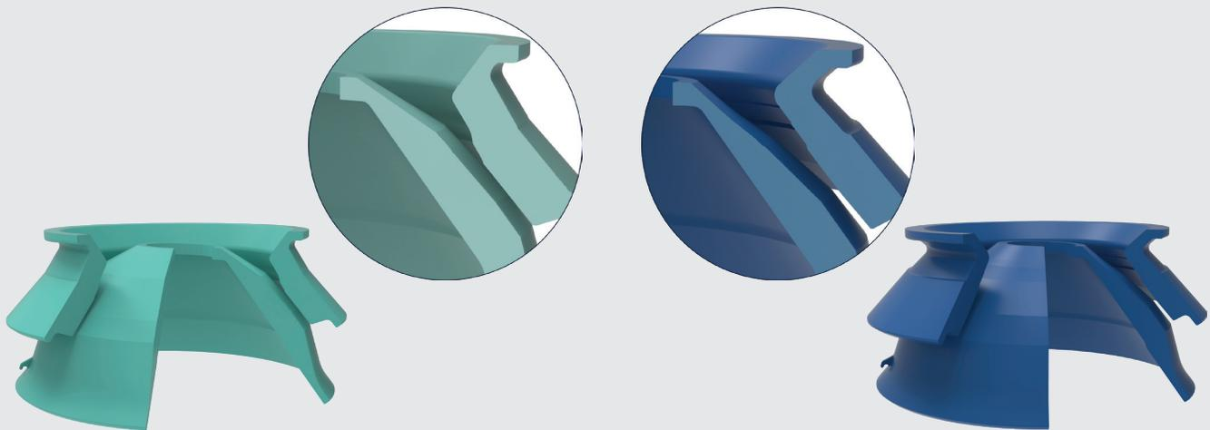
The previous liner design was not able to maintain the necessary CSS during operation and the liners were removed before being fully worn out.
