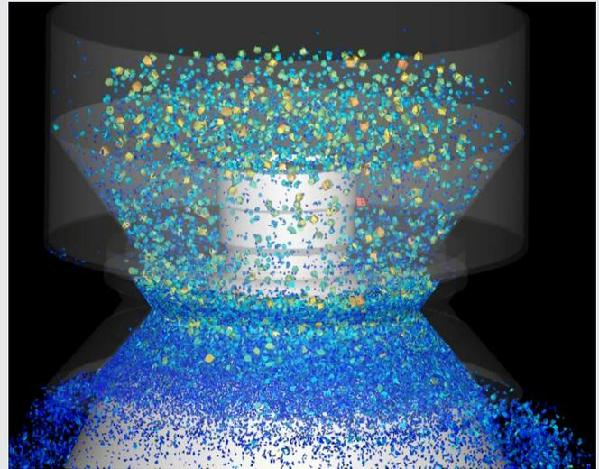
Performing a discrete element method (DEM) analysis of the crusher liners to ensure optimal performance
