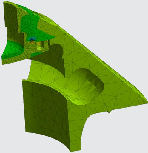
Stress analysis of the crusher component to optimise design
