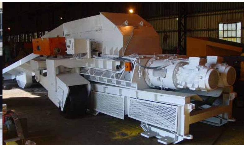
Underground Feeder Sizer Combination
