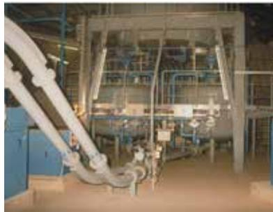
Double pressure vessel with pre-hopper
